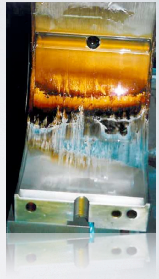
Varnish deposit in bearing
